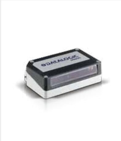
The DS1100 embedded bar code reader is a cost-effective laser scanner characterized by ultra-compact dimensions, motor on/off software commands, wide reading width at a short reading distance, lightweight design (<100 g), built-in RISC decoder, scanning speed of 500scans/sec, dual high speed serial interface, and IP65 rugged industrial housing.
